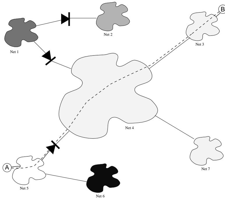
Figure 3.15: Tunneling past a firewall.
