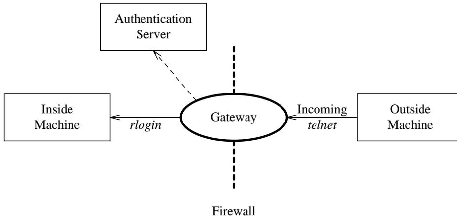
**Figure 3.14:** Call flow diagram for incoming *telnet* access.
