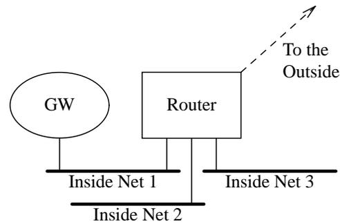
**Figure 3.9:** A firewall router with multiple internal networks.
