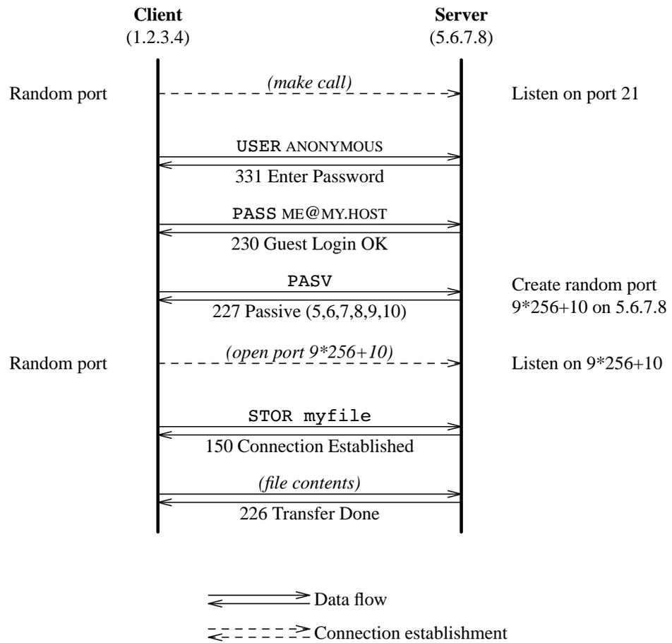
Figure 3.5: Using FTP with the PASV command.
