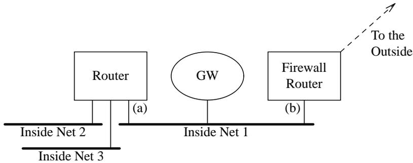
**Figure 3.10:** A firewall with output-filtering routers.
