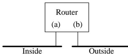
Figure 3.8: A typical firewall router.
