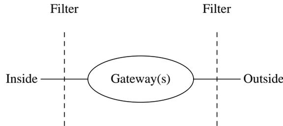
**Figure 3.1:** Schematic of a firewall.
